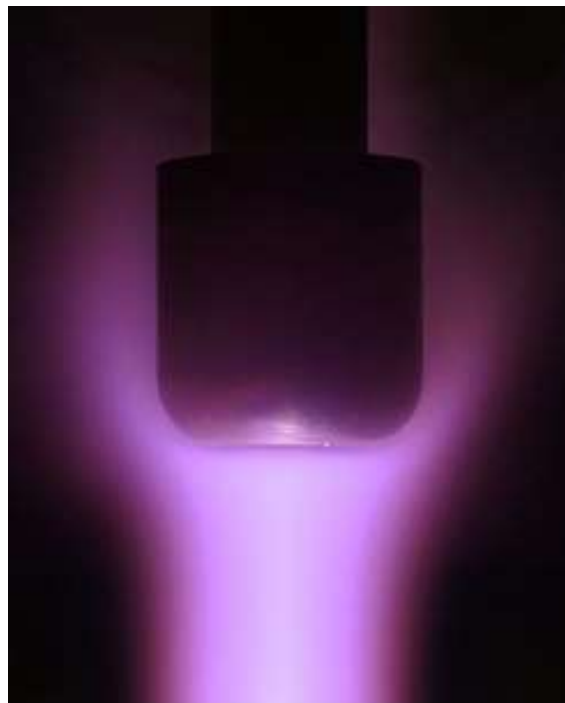
Flow around the blunt face model (probe) with rounded edge in the subsonic jet of dissociated air in the test chamber of VGU-4 HF induction plasmatron
