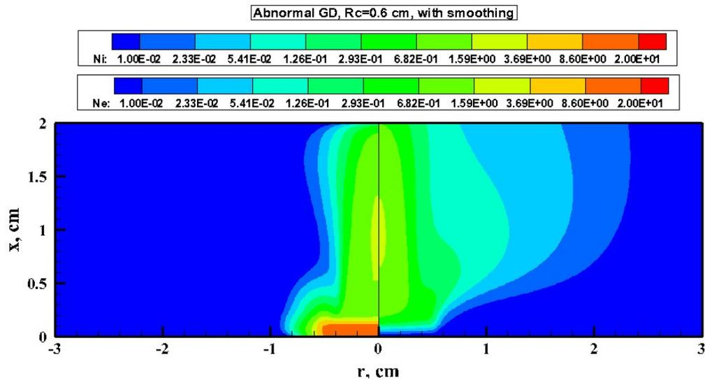
Distributions of the ion (left) and electron (right) concentrations in a normal glow discharge,  $\varepsilon=1000$  V,  $R_0=300$  k $\Omega$ ,  $p=5$  Torr. Radius of the cathode section  $R_c=0.6$  cm. Calculation with smoothing of the electric field near the cathode
