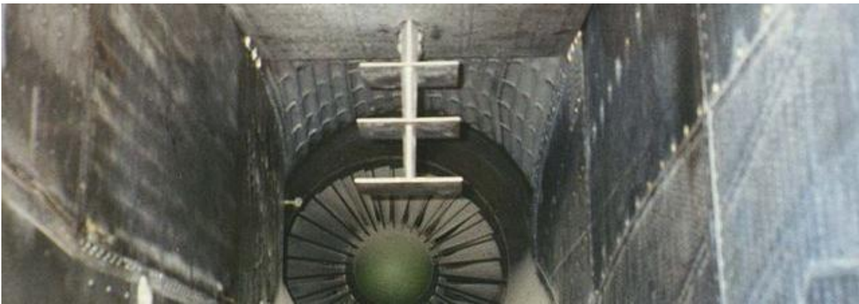
Fig. 2. The water-methanol vaporizer in the inlet of the MIG-25.
